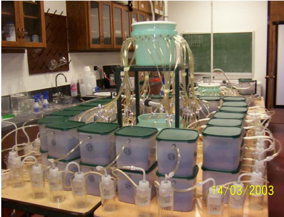
Figure 1. Photograph of the ammonia emission apparatus consisting of Tupperware® air emission chambers and acid traps connected to a vacuum pump.
